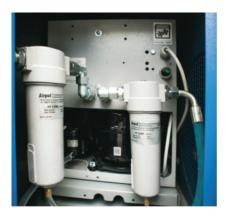
Prefilter – high porosity of the nonwoven fabric, which the filter element is made of, ensures high ability to store dust. It guarantees removal of 99% of solid particles larger than 3 µm.
