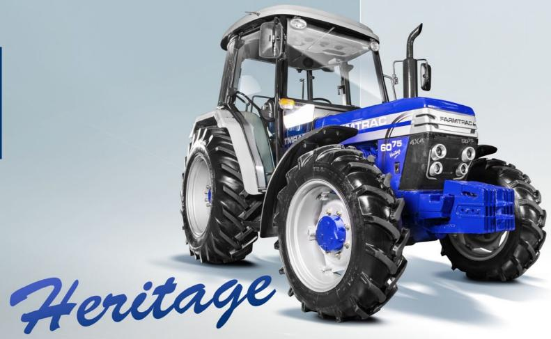
The Heritage tractors are compatible (robust front axles) with front loaders with a lift capacity exceeding 1200kg. As these tractors are characterized by high weight (about 3t) they have a high pulling power. These reliable engines are fuel efficient and use only 4 l/h when operating a front loader.
